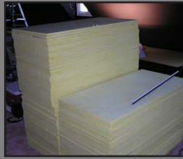
Sound Absorption Core, 1"-4" Thick
